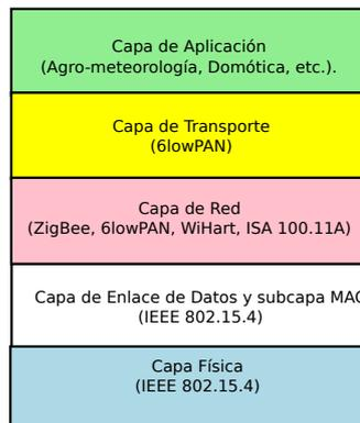
Figura 2.3: Pila de Protocolos WSNs. Figura basada en [Zheng and Jamalipour, 2009].
